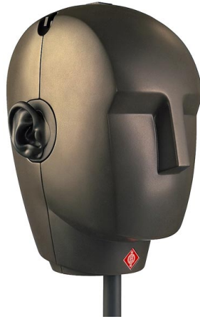
Figure 5: An example of the dummy head used in measuring HRTFs [8].
