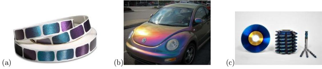
Figure 7: Color shifting ink changes its color depending on the viewing angle. Selected examples include color shifting ink, used (a) against counterfeit [17], (b) for decoration [18], and (c) on machine parts to help spot mechanical damage [19].
