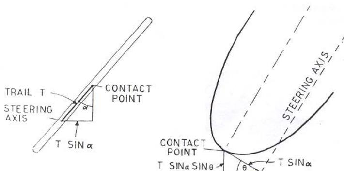
Figure 6. Top view of the front wheel (left). As the bicycle is steered, the front wheel rotates about the contact point, moving the bicycle sideways a distance  $T \sin \alpha$ , where  $T$  is the trail (left). Front view of front wheel (right). For a leaning bicycle this creates a vertical displacement of  $H = T \sin \alpha \sin \theta$ . The frame of the bicycle is perpendicular to the plane of the paper [3].
