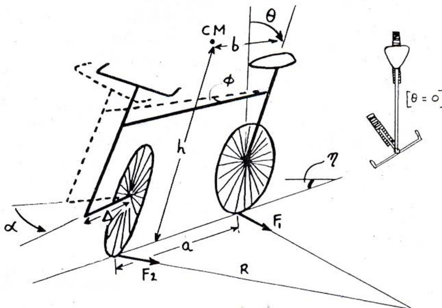
Figure 7. Sketch of simplified bicycle showing the parameters important in the analysis of bicycle stability. CM is the center of mass of the bicycle with rider.  $R$  is the radius of the bicycle's path [4].
