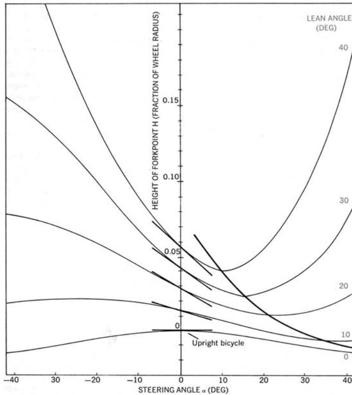
Figure 3. Plot of steering angle versus height of forks for different lean angle. Minimal height or the lowest potential energy occurs closer to straight-ahead position for higher values of lean angle. The tich line connects the minima at different lean angle [2].
