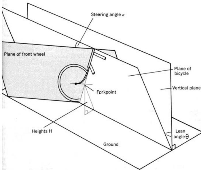
Figure 2. Sketch of leaning bicycle and definition of the steering angle  $\alpha$  and the angle of lean  $\theta$  [2].
