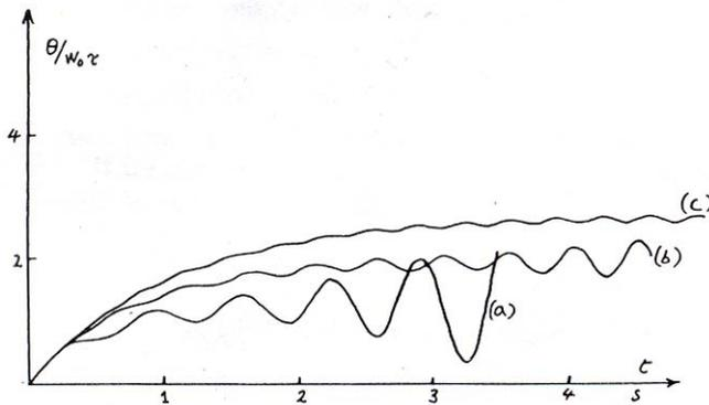
**Figure 10. Solutions for leaning angle with different castors as measured by the parameter  $\mu$ . Curve (b) is the predicted response of a real bicycle. Curve (a) shows the predicted response if the castor were halved ( $\mu = 66.5 \text{ s}^{-2}$ ), and curve (c) is the prediction for twice the castor ( $\mu = 266 \text{ s}^{-2}$ ). Speed is 5 m/s [4].**
