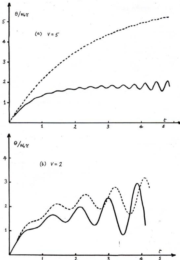
Figure 9. Influence of gyroscopic effect of the front wheel on bicycle stability. The dotted curves is a simulation without gyroscopic effect and the solid curves is a simulation with gyroscopic effect. The gyroscopic effect is stabilizing in the sense that result in a smaller mean value of  $\theta$ , but destabilizing in the sense that it enhances the oscillatory instability. Curve (a) speed 5 m/s; (b) 2 m/s [4].
