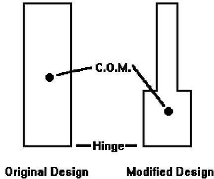
Fig. 9: The way of moving the centre of mass (com) closer to the hinge<sup>8</sup>.
