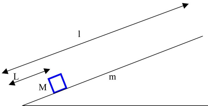
Fig. 10: The small weight fastened on the stick near the hinge will enhance the acceleration of the end of the stick.  $M$  – mass of the weight,  $m$  - mass of the stick,  $L$  – distance from hinge to the weight,  $l$  – length of the stick
