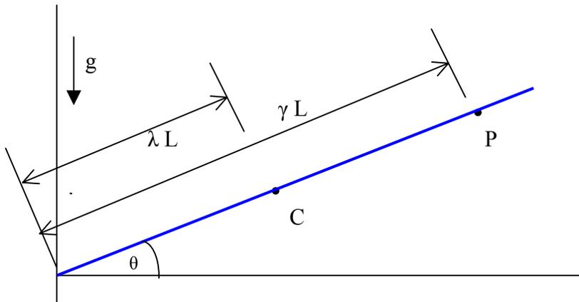
Fig. 4: Geometry of a falling stick of length  $L$  and mass  $M$ . Point C denote centre of mass, and point P denote position of the particle with mass  $m$ .
