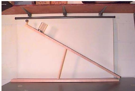
Fig.1: Demonstration of a "faster than gravity" fall called falling chimney<sup>2</sup>
