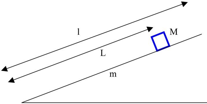
Fig. 7: The small weight fastened to the free end of the stick will reduce the acceleration of the end of the stick.  $M$  – mass of the weight,  $m$  - mass of the stick,  $L$  – distance from hinge to the weight,  $l$  – length of the stick
