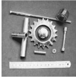
*Figure 22:* Zr-based BMGs in different shapes.
